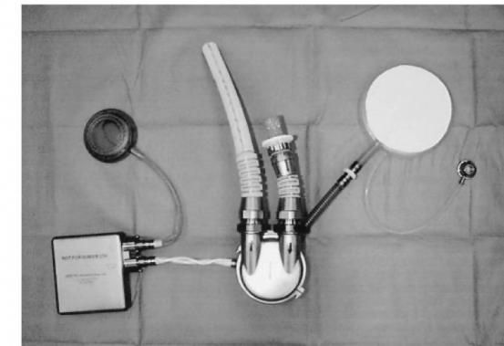
Fig 1. Components of the LionHeart LVS-2000 including the motor controller, pump assembly, and compliance chamber.
